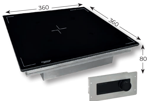
Product cut-out dimensions: 366 x 366 mm Control panel cut-out dimensions: 215 x 88mm
